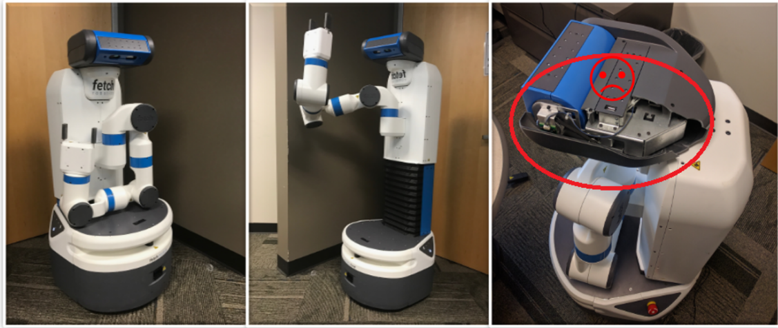
Figure 4.1: The Fetch in the Crouched Position with Arm Tucked (Left), Torso Raised and Arm Outstretched (Middle) and the Rather Tragic Consequences of a Mistaken Action Model (Right Showing a Fractured Head from an Accident).
